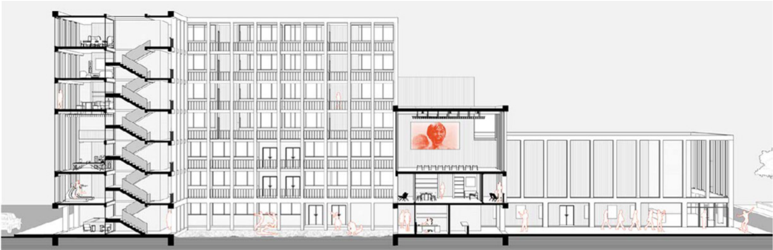
Longitudinal section / stepped volumes and vertical circulation
